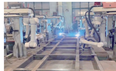
Steel Frame Welding
